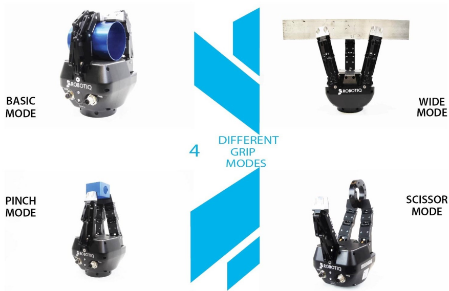
Figure 1.3 : The four Operation Modes of the 3-Finger Adaptive Robot Gripper.
