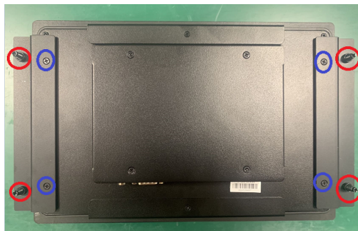
Figure 2.14 Install panel mount bracket
