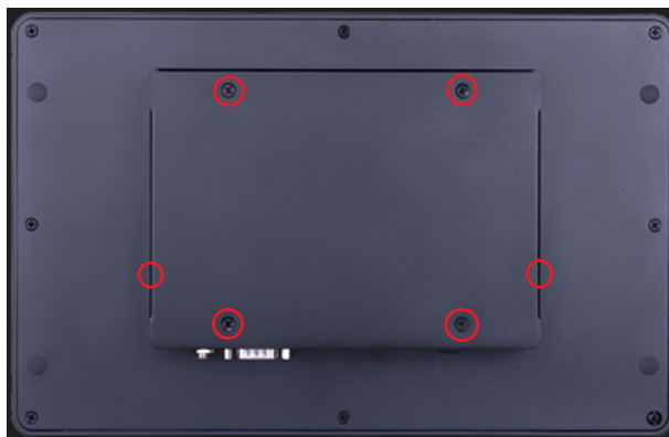
Figure 2.3 Retention screws on rear cover
