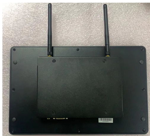
Figure 2.7 Location of external antenna
