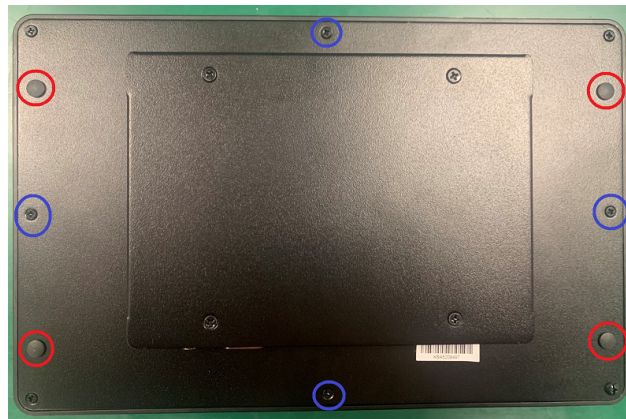
Figure 2.18 Remove rear cover
