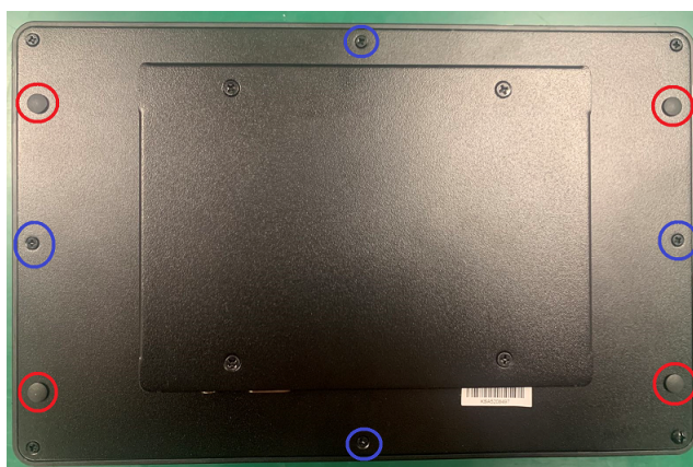
Figure 2.12 Remove rear cover
