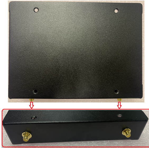
Figure 2.5 Antenna cable assemble on rear cover
