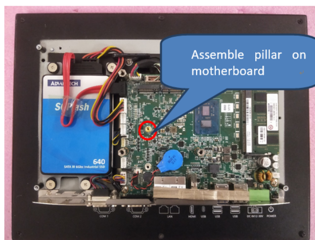
Figure 2.12 Install the Pillar on the Motherboard
