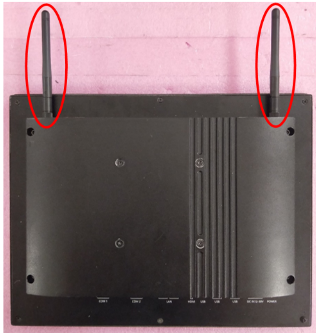
Figure 2.17 Assemble the Wi-Fi Antenna
