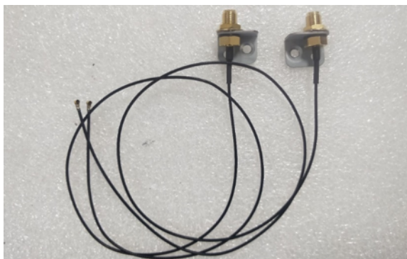
Figure 2.15 Assemble the Bracket with the Antenna Cable
