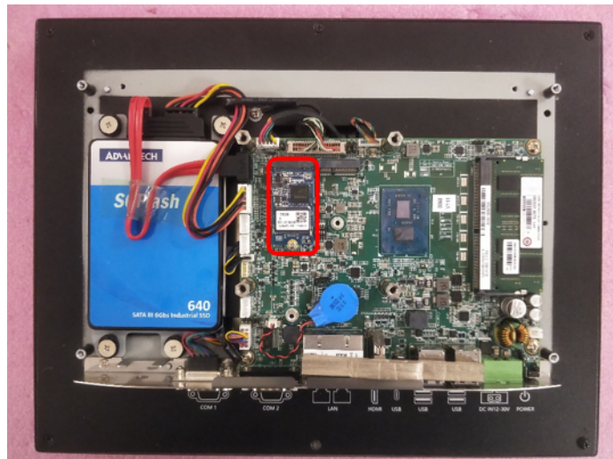
Figure 2.13 Install the M.2 2242 Card on the Motherboard
