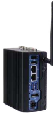
Install the antenna
