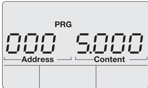
Fig. 20.1 “Programming Mode” display example, address 000 with content 5,000.
